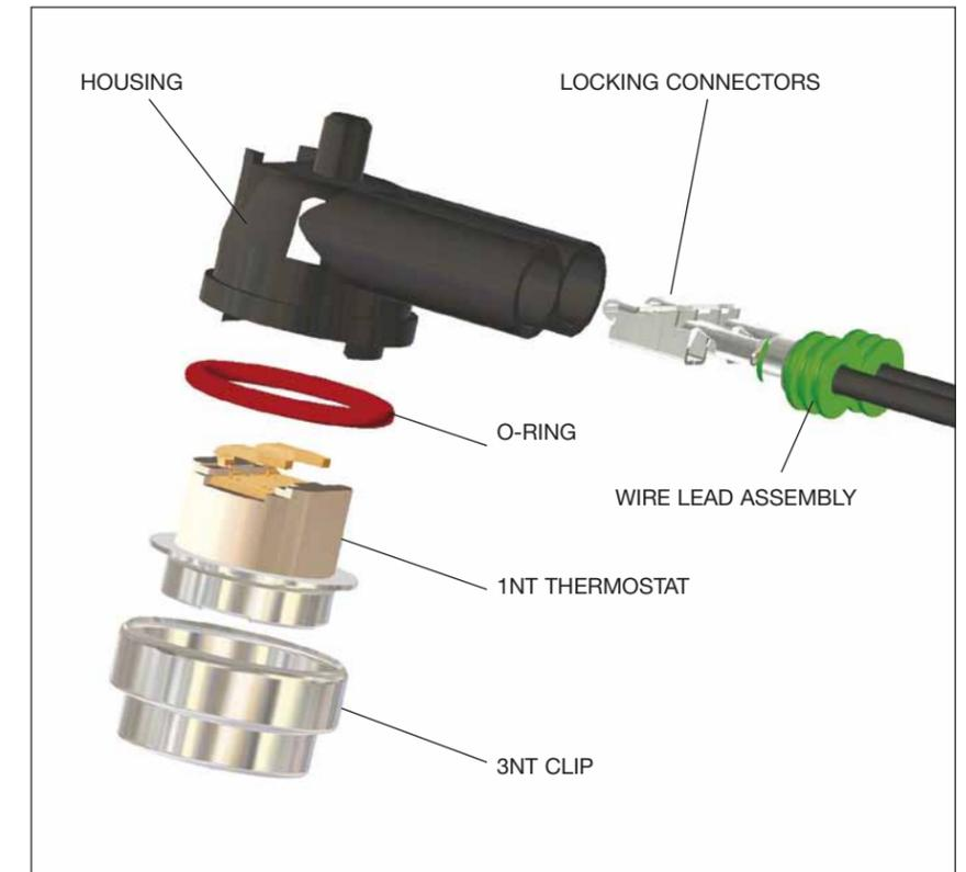
**Important Notice:** The 3NT is not hermetically sealed, and should not be submerged in liquid. For such applications, please contact Sensata Technologies for advice.
