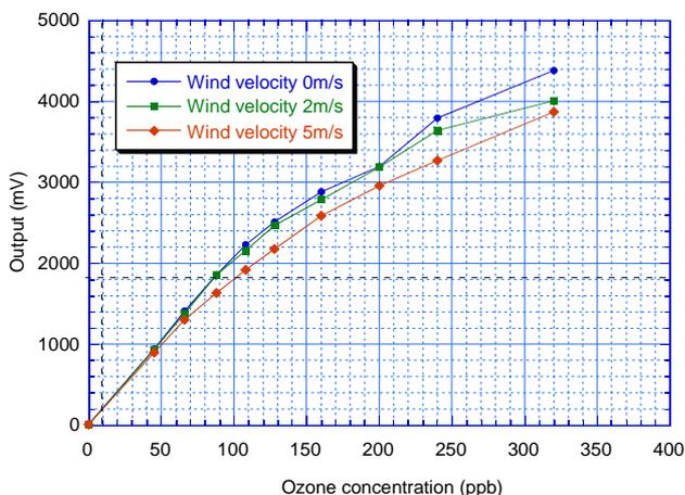
Fig. 5 Wind influence (Output range: 1 to 5V)
