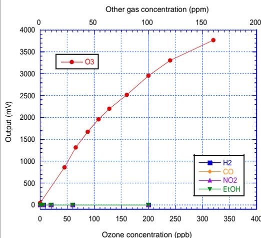
Fig. 3 Monitor sensitivity characteristics (Output range: 1 to 5V)
