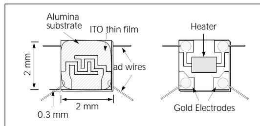
Fig. 1 Sensing Elements
